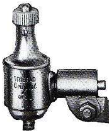
b) AlNi-Magnet 8-polig 1953--1957
