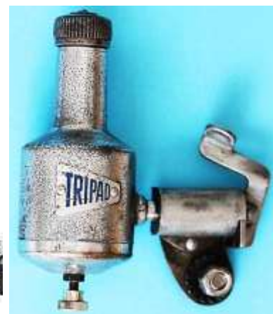
c) Keramikmagnet 8-polig 1963
