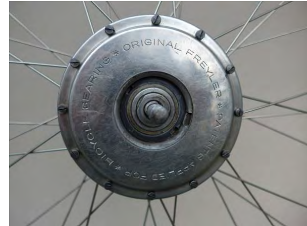
Freyler decorated cover with sun gear shifting hole at 4 o'clock
