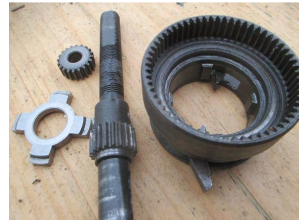
Sturdy and compact Sturmey Archer planet, sun and ring gear to compare
