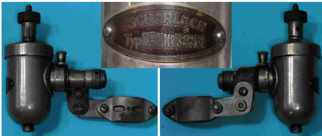
Bild.1.8: Scharlach F No. 65/5, rotierender Magnet
