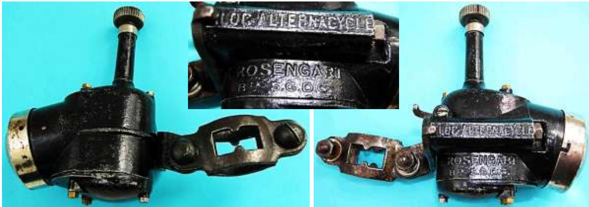
Bild 3.1: Dynamo-Lampen-Kombination: Bloc. Alternacycle, Rosengart, Paris
